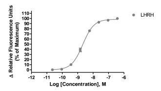
Figure 1. Representative data for activation of GnRH receptor. Calcium flux in GnRH–expressing Chem-1 cell line induced by LHRH. GnRH–expressing Chem-1 cells were loaded with a calcium dye, and calcium flux in response to the indicated ligand(s), 4-fold serial dilution with each concentration performed in duplicate, was determined on a Molecular Devices FLIPR<sup>TETRA</sup>. Maximal fluorescence signal obtained in this experiment was 4,600 RLU (Relative Light Units).
